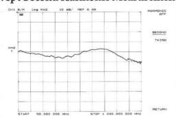
In this example, changing the reference position to the top of the screen [SCALE REF], [REFERENCE POSITION] [1] [0] [x1] will let us view the fundamental and harmonic responses on the same display.
