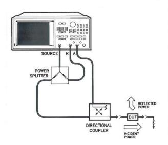
Reflection measurements require a directional device, such as a directional coupler, in the measurement setup. This signal separator provides a sample of the power traveling in one direction only. For reflection measurements it is connected as shown in the figure, allowing the power reflected from the DUT to be separated and measured independently of the incident power. The ratio of these two signals is the reflection coefficient of the DUT or, when expressed in decibels, the return loss.
