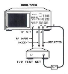
Analyzer and Test Set Connections
