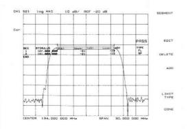
Determine pass or fail status by comparing the device performance to limit lines on the display. In the example, a flat limit line lets you quickly make GO/NO GO testing decisions regarding the filter's pass band ripple by comparing the measurement trace to the limit lines on the display.
