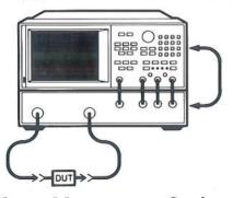
Insertion loss and gain are ratios of the output to input signals. When set up as shown below, the results can be read directly in decibels.
