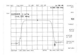
The wide dynamic range of the HP 8753C allows it to measure stopband rejection up to 110 dB below the pass band response. As discussed in chapter 6, "Increase Dynamic Range", maximum dynamic range requires proper selection of input power level, IF bandwidth and averaging.
