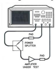
Measurements to this point have all been made with a constant input amplitude and swept test frequency range. At times, however, it may be desirable to characterize a device at a single frequency as a function of input amplitude. By using the power sweep mode, measurements such as gain compression or AGC (automatic gain control) slope can be made.
