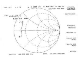
The display shows the complex impedance of the DUT over the frequency range selected. Press [MKR] and use the knob to read the resistive and reactive components of the complex impedance at any point along the trace. Note that the marker annotation tells that the complex impedance is capacitive in the bottom half of the Smith chart display and is inductive in the top half of the display.
