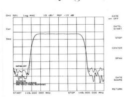
Time domain analysis also lets you mathematically remove individual parts of the time domain response to see the effect of potential design changes. We do this by "gating" out the undesirable responses. In the example shown to the left we see the effect of removing the RF leakage and the triple travel signal path using gating. By transforming back to the frequency domain we see that this design change would yield better out-of-band rejection for the SAW filter under test.
