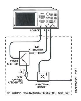
While simple transmission and reflection measurement setups can be constructed from discrete RF components such as power dividers, directional bridges, cables, attenuators, etc., it is easier to use an integrated test set such as the HP 85044A/B transmission/reflection test set.
