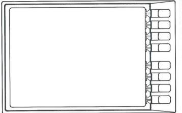
One of the more noticeable characteristics of the HP 8753C is the simplicity of its front panel. Rather than individual keys for each of the many instrument functions, the analyzer uses CRT-displayed "menus" for operator input. These menus list the possible choices for a particular function, with each choice corresponding to one of the eight "softkeys" located to the right of the CRT.
