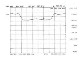
To display the same data in terms of reflection coefficient, press **[FORMAT]** *[LIN MAG]*. This simply redisplays the existing measurement in a linear magnitude format that varies from  $\Gamma=1.00$  at the top of the display (100% reflection) to 0.00 at the bottom of the display (perfect match).
