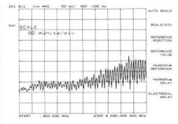
The figure shows the frequency domain reflection response of the cables under test. The complex ripple pattern is caused by reflections from the adapters interacting with each other. By transforming this data to the time domain, you can determine the magnitude of the reflections versus distance along the cable.
