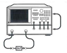
to the mechanical "line stretchers" of earlier analyzers. This feature simulates a variable length loss less transmission line, which can be added to or removed from a receiver's input to compensate for interconnecting cables, etc. In this example, the electronic line stretcher is used to measure the electrical length of a test device.
