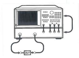
Connect the S-parameter test set to the analyzer as shown. The DUT will be the SAW filter used previously.
