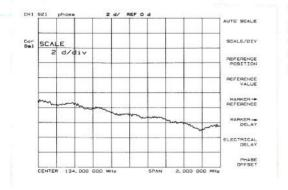
This can be measured using the previous setup for measuring electrical length. By adding electrical length to "flatten out" the phase response we have removed the linear phase shift through the DUT. What remains is the deviation from linear phase shift through the device. Simply increase the scale resolution to directly measure the deviation from linear phase.
