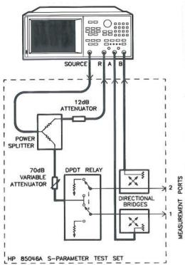
The S-parameter test set contains the hardware required to make simultaneous transmission and reflection measurements in both the forward and reverse directions. The only setup required is to connect the DUT to the two measurement ports. The network analyzer controls the switching functions, so that even reverse measurements can be made without changing device connections. The internal switch simplifies full 2-port measurement calibrations.
