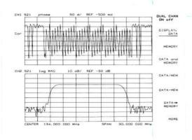
In some cases it is useful to be able to view more than one measured parameter at a time. Simultaneous gain and phase measurements for example, are useful in evaluating stability in negative feedback amplifiers. Such measurements are easily made using the dual channel display.
