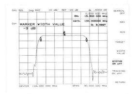
The HP 8753C calculates the bandwidth of the DUT between two equal power levels. In this example, we calculate the -3 dB bandwidth relative to the filter center frequency.
