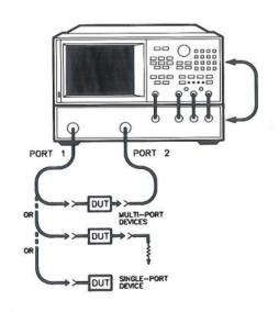
These parameters are really no different from the measurements made in the previous section.  $S_{11}$  is the complex reflection coefficient of the DUT input, while  $S_{22}$  is the complex reflection coefficient of the DUT output. In both cases, all unused ports must be properly terminated.
