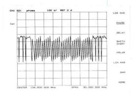
Press [LOCAL] [SYSTEM CONTROLLER] [SAVE] [STORE TO DISK] [STORE FILE nn] to store the result (data trace, measurement settings, and calibration) on an external disk. (See the "Disk Drive" tutorial for details.) Or just observe the trace.
