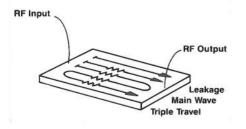
In the example in chapter 3, the transmission response of a SAW filter is measured. The inverse Fourier transform of that transmission measurement is also shown. Note the three components of the transmission response: RF leakage at near zero time, the main travel path through the device (1.6  $\mu s$  travel time) and the "triple travel" path (4.8  $\mu s$  travel time). Each of these signal paths illustrated in the diagram to the left.
