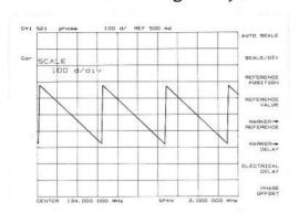
The above setup results in the phase response measurement shown. Note that the SAW filter under test has considerable phase shift within only a 2 MHz span. Other filters may require a larger frequency span to see the effects of phase shift.
