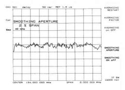
The phase linearity of many devices is specified in terms of group or envelope delay. This is especially true of telecommunications components and systems.
