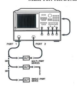
Reflection measurements are made with only one port of a test device. But when the device has more than one port, care must be taken to insure that the unused port(s) are properly terminated in their characteristic impedance (e.g. 50 or 75 ohms). If this is not done, reflections off the unused ports will cause measurement errors.
