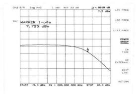
The figure shows the gain rolling off as the input power increases to a level where the amplifier under test exhibits gain compression. While the  $\pm 20$  dBm maximum output from the network analyzer will be sufficient for many compression tests, it is also possible to add an external amplifier in series with the source to provide additional drive. Remember to limit the input power to the analyzer to 0 dBm maximum, adding external attenuators if necessary.
