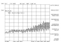
To transform to the time domain press [SYSTEM] and [TRANSFORM MENU]. Select [BANDPASS] transform mode. The low pass impulse mode is most similar to the TDR but we use the bandpass mode in this example because it is simpler. Refer to the "Reference" section of the Operating Manual for a complete description of all the time domain operating modes.
