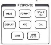
The network analyzer's receiver section is controlled with these keys. The top three keys allow the user to choose measurement configuration (A, B, B/R, etc.), presentation format (amplitude and phase versus frequency, Smithchart, polar coordinates, etc.), and scale and reference values for a full screen display.
