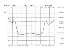
To display the reflection measurement data in terms of standing wave ratio (SWR), press **[FORMAT]** [SWR]. The analyzer reformats the display in the unitless measure of SWR with SWR = 1 (perfect match) at the bottom of the display.
